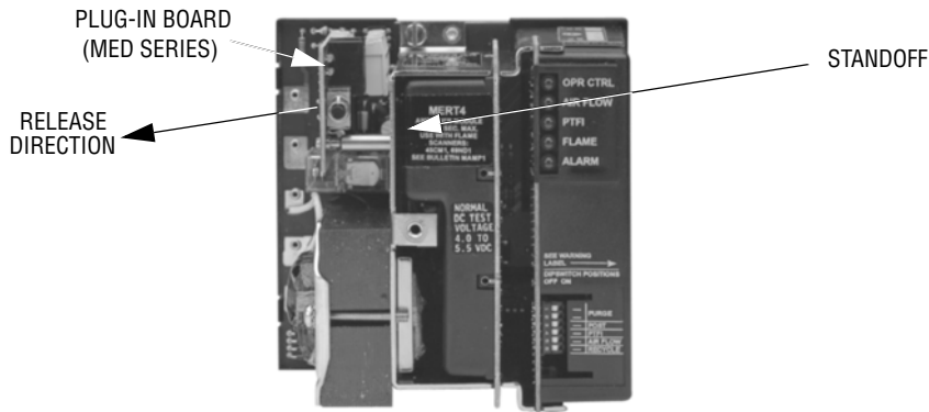
FIGURE 4. PLUG-IN BOARD LOCATION AND INSTALLATION
